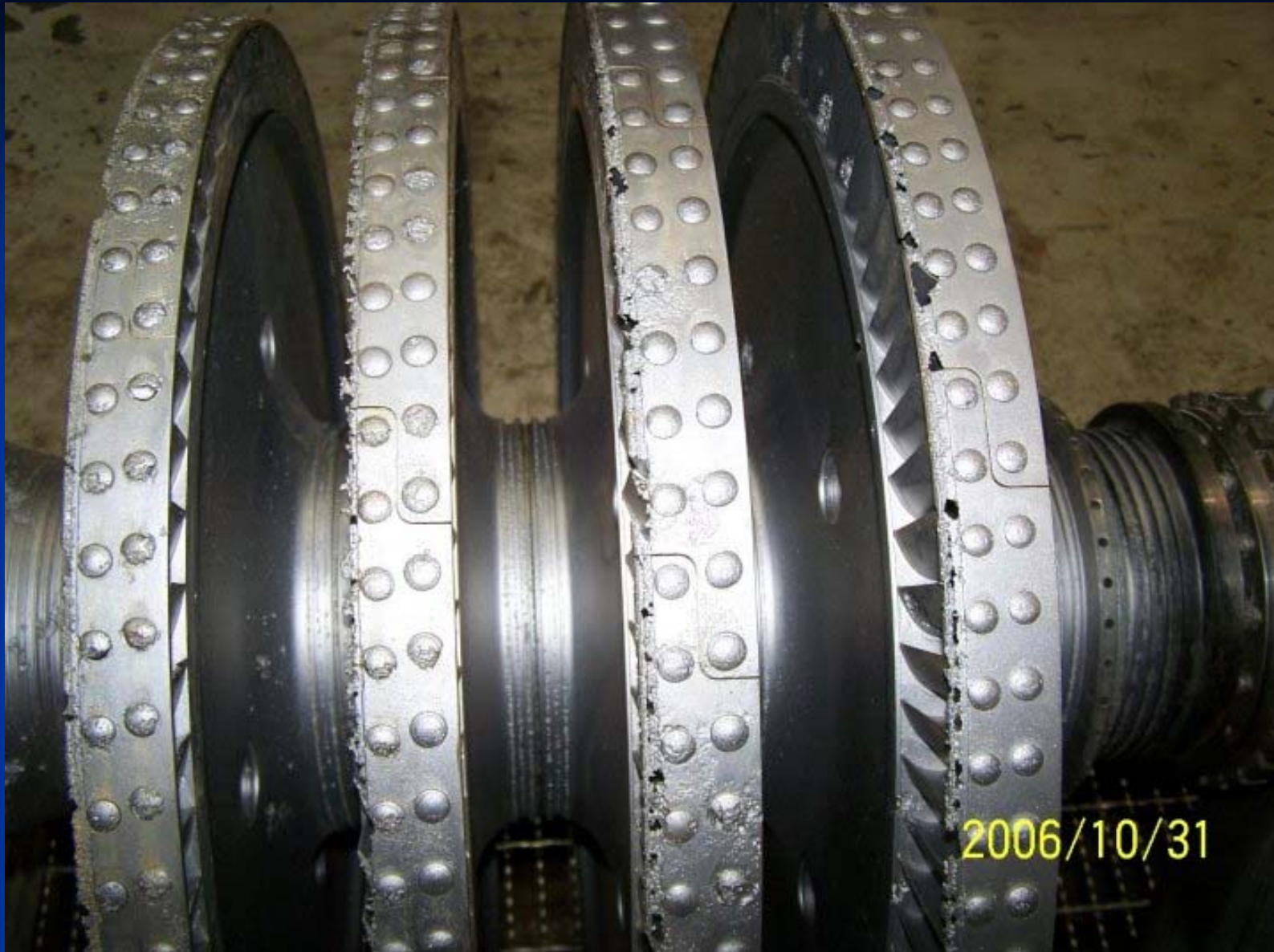
Corroded shroud bands
